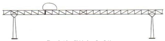
Figure 5. A Low Weight, Low-Cost Guideway
