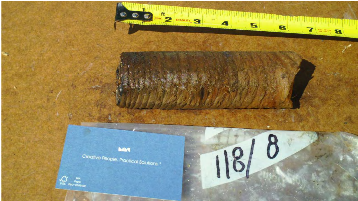
Photo 1-5: Typical Core (From Pile 8 on Bent 118)
