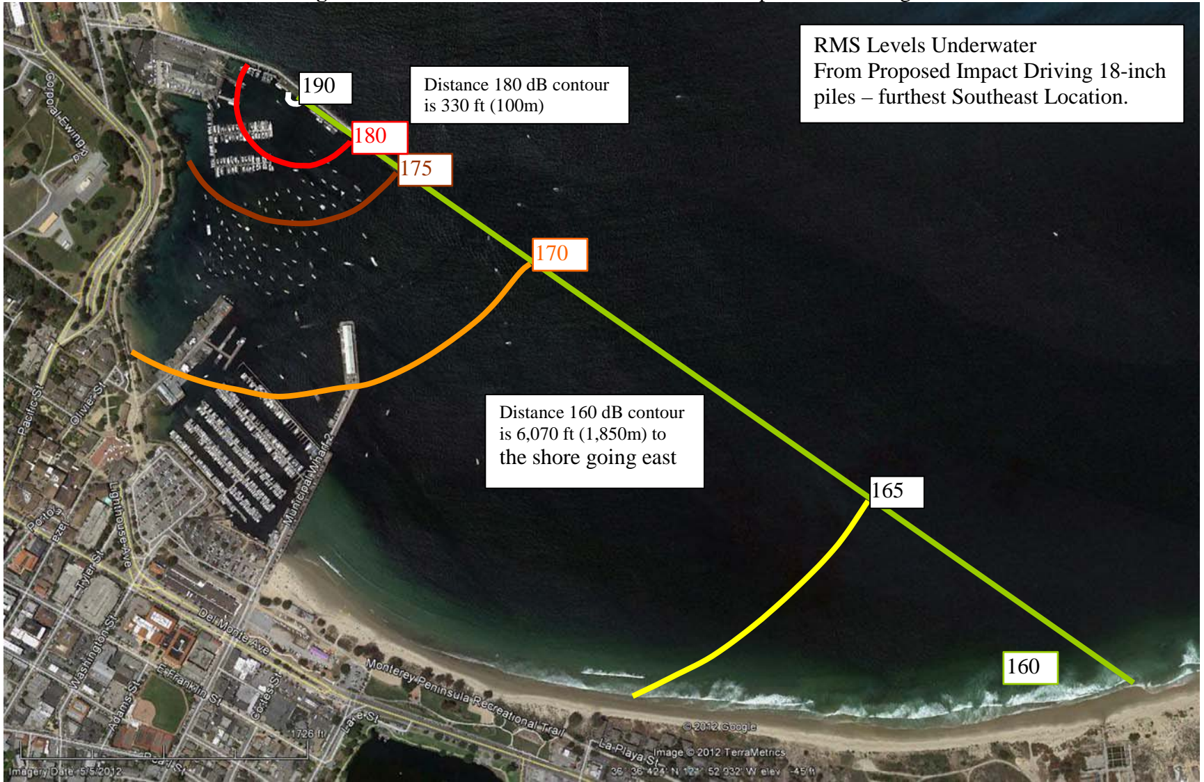
Figure 5. Extent of RMS Sound Pressures from Impact Pile Driving
