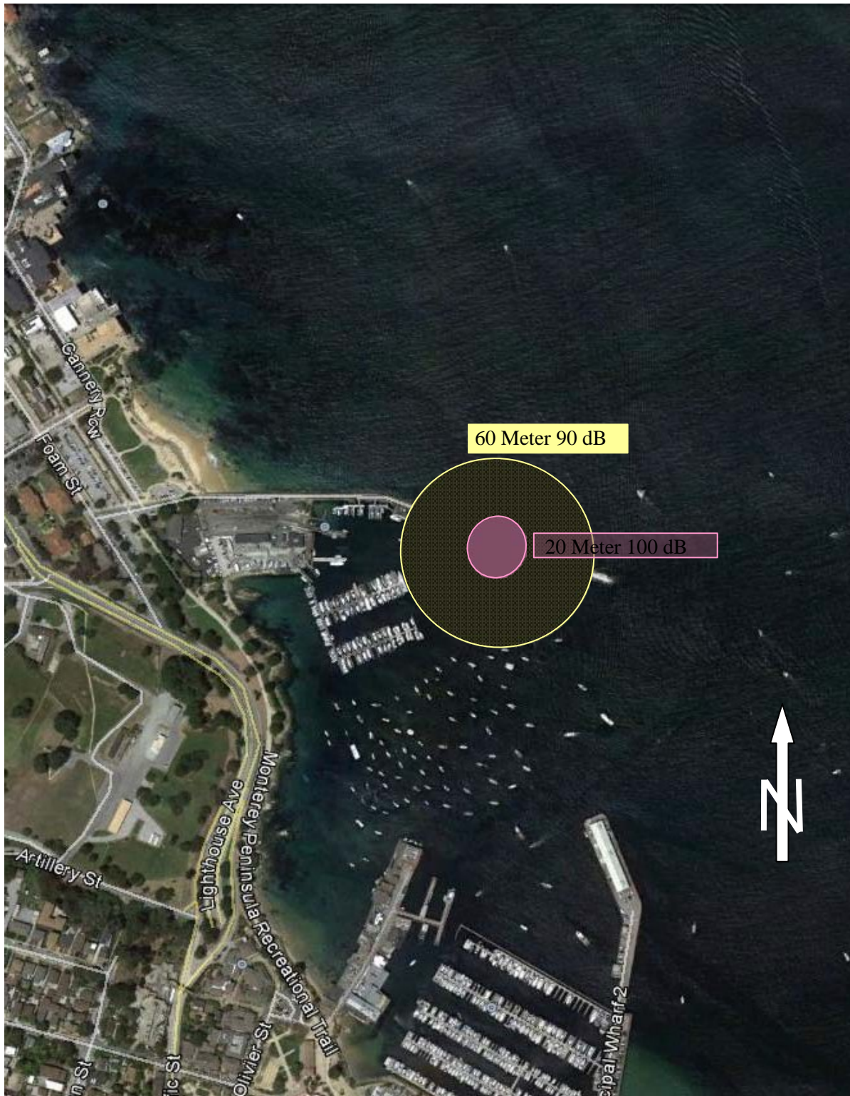
Figure 6. Extent of Airborne L_{max} Sound Levels from Vibratory Pile Driving
