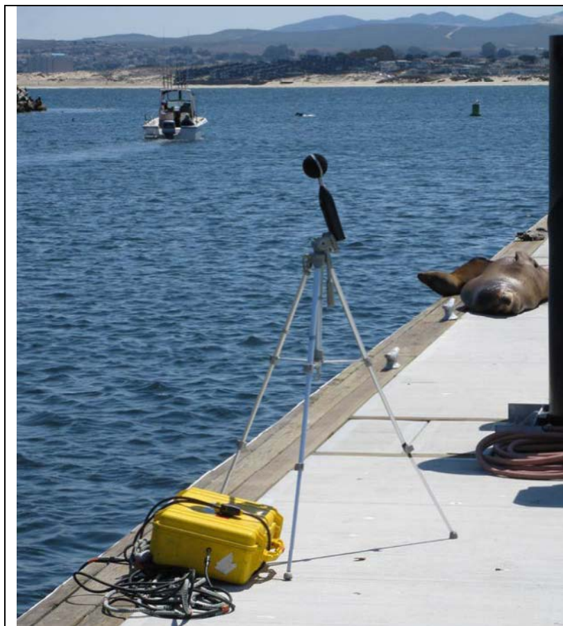
Figure 10. Airborne and underwater acoustic monitoring at new dock across from USCG pier.
