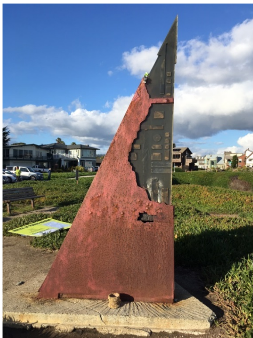
Effects of the marine air and spray have pitted and rusted the piece.
