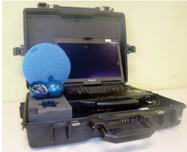
Figure A1.1. SmartBall Core, Foam Shell, and SmartBall Receiver (SBR).
