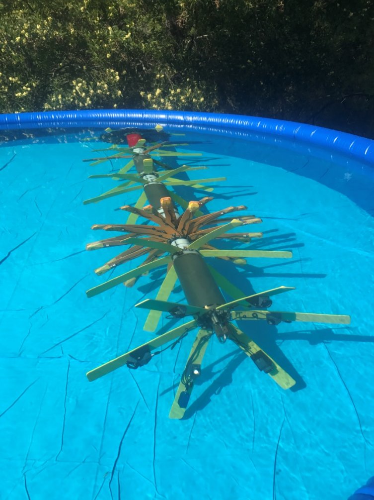
Days 2-4 - "PipeDiver" (electromagnetic inspection device)
