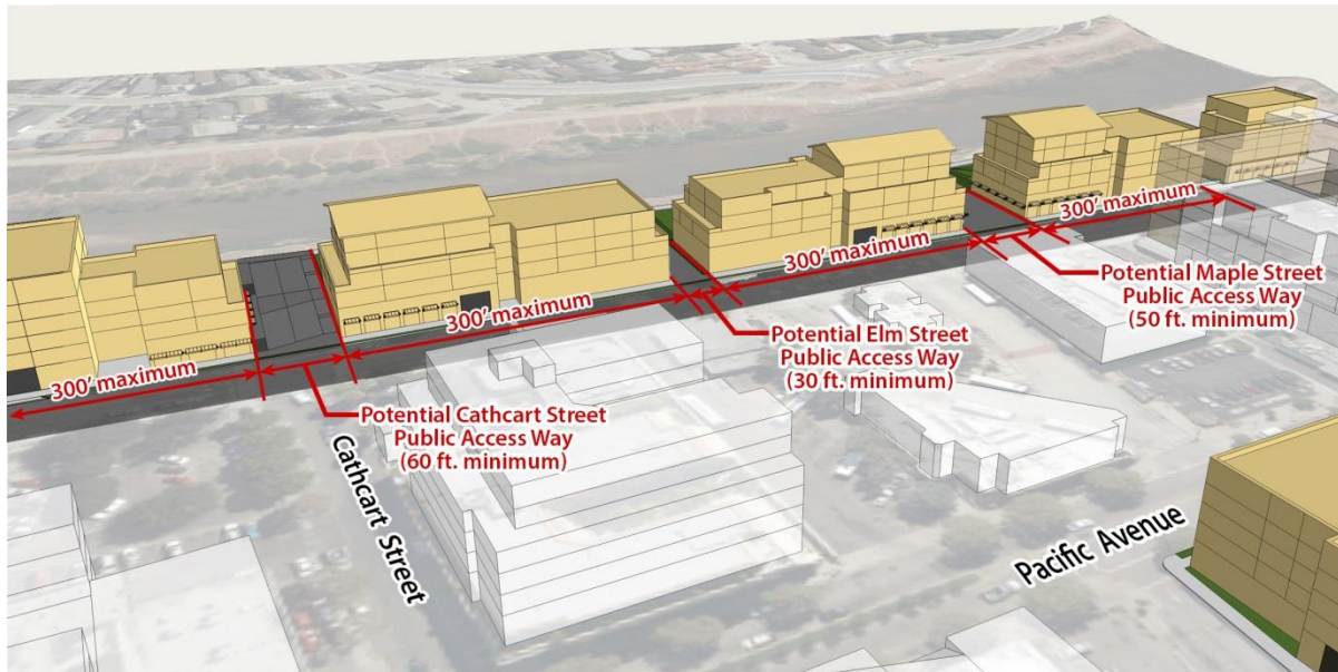
Figure E-2: Proposed building massing and public access requirements along Front Street and the riverfront.
