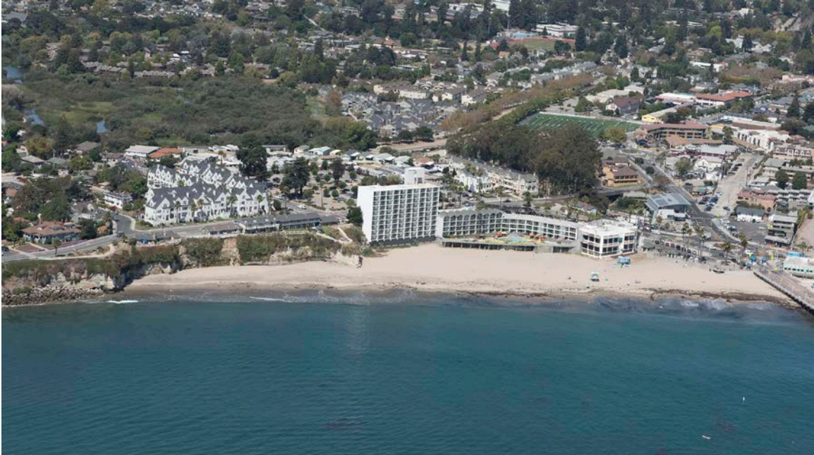
Figure 2. Wide sandy beach fronting Dream Inn. Note rip-rap and lack of beach immediately to the left (upcoast). (2015 photo from California Coastal Records Project)
