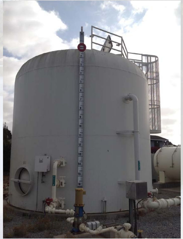
Beltz 12 Volumetric Meter Accuracy Testing
