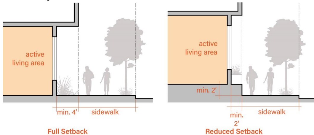
Figure 16: Ground Floor Residential – Without Individual Access
