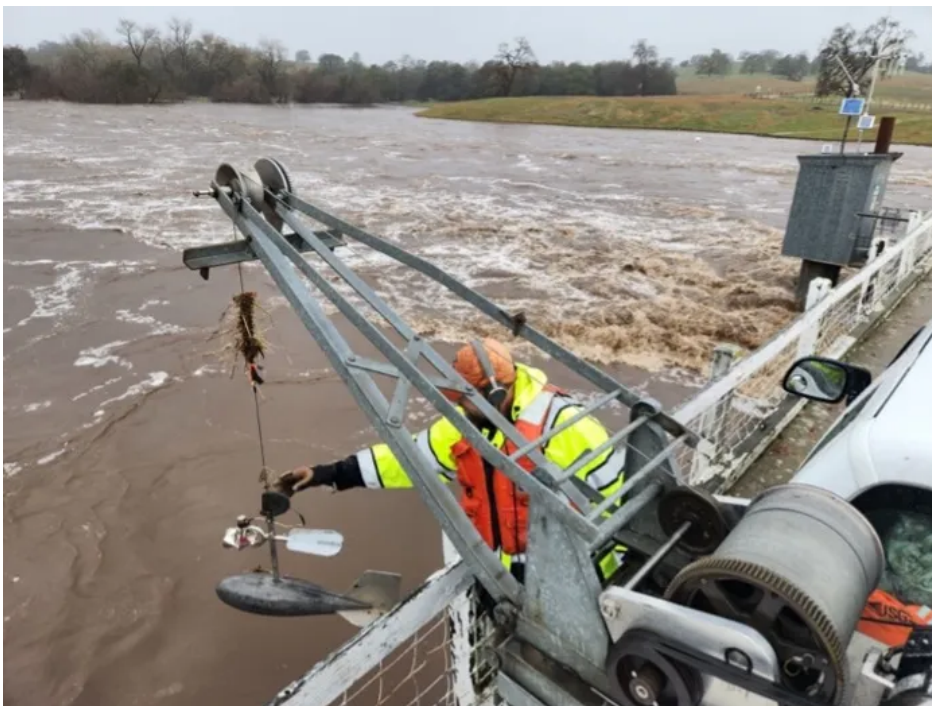
Travis Hiett of USGS measures high flows on the Cosumnes River, December 31, 2022, from the bridge at Michigan Bar. Flows were estimated at 63,700 cfs.
