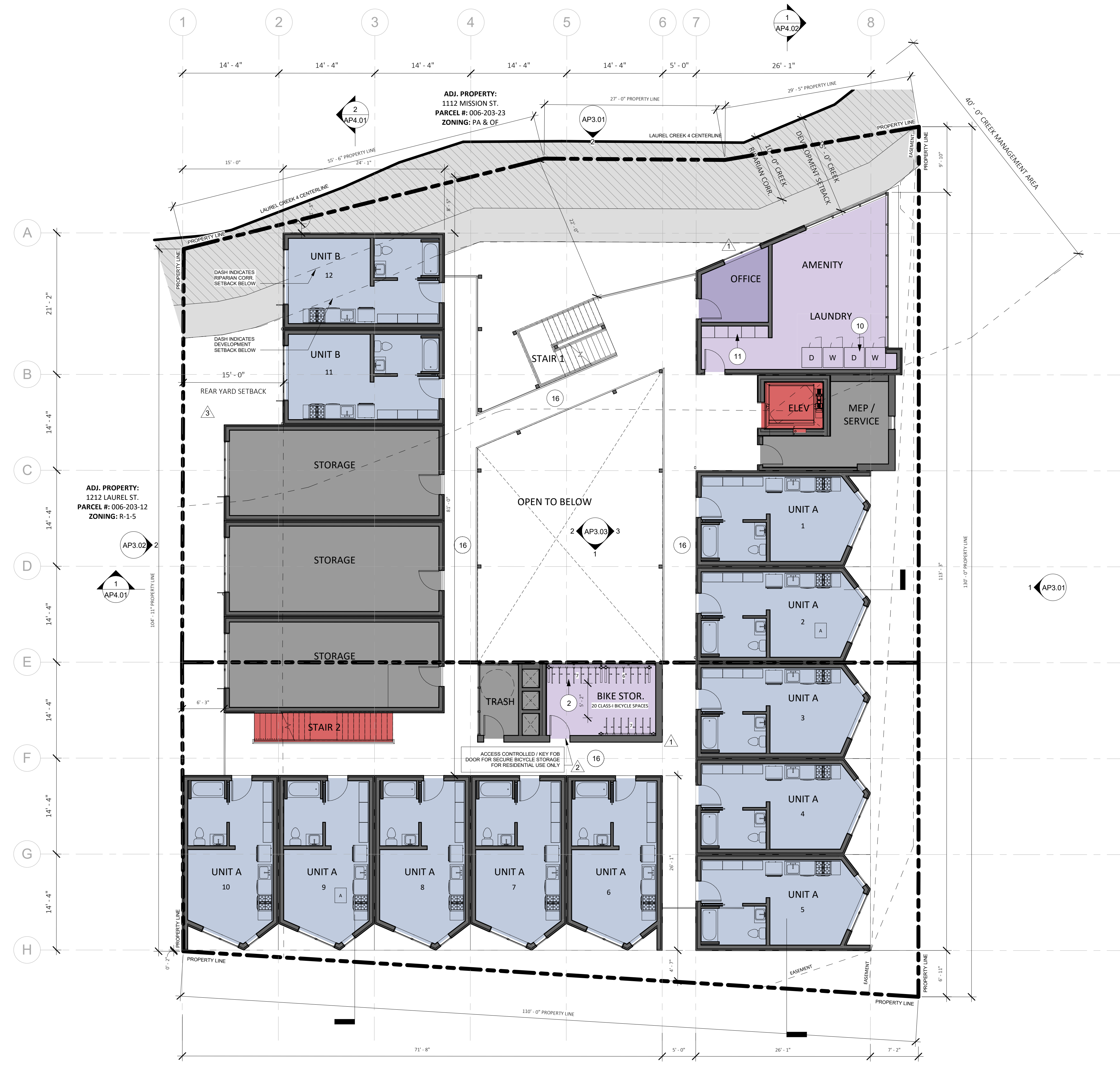
1 PROPOSED FLOOR PLAN - LEVEL 3 1/8" = 1'-0"
