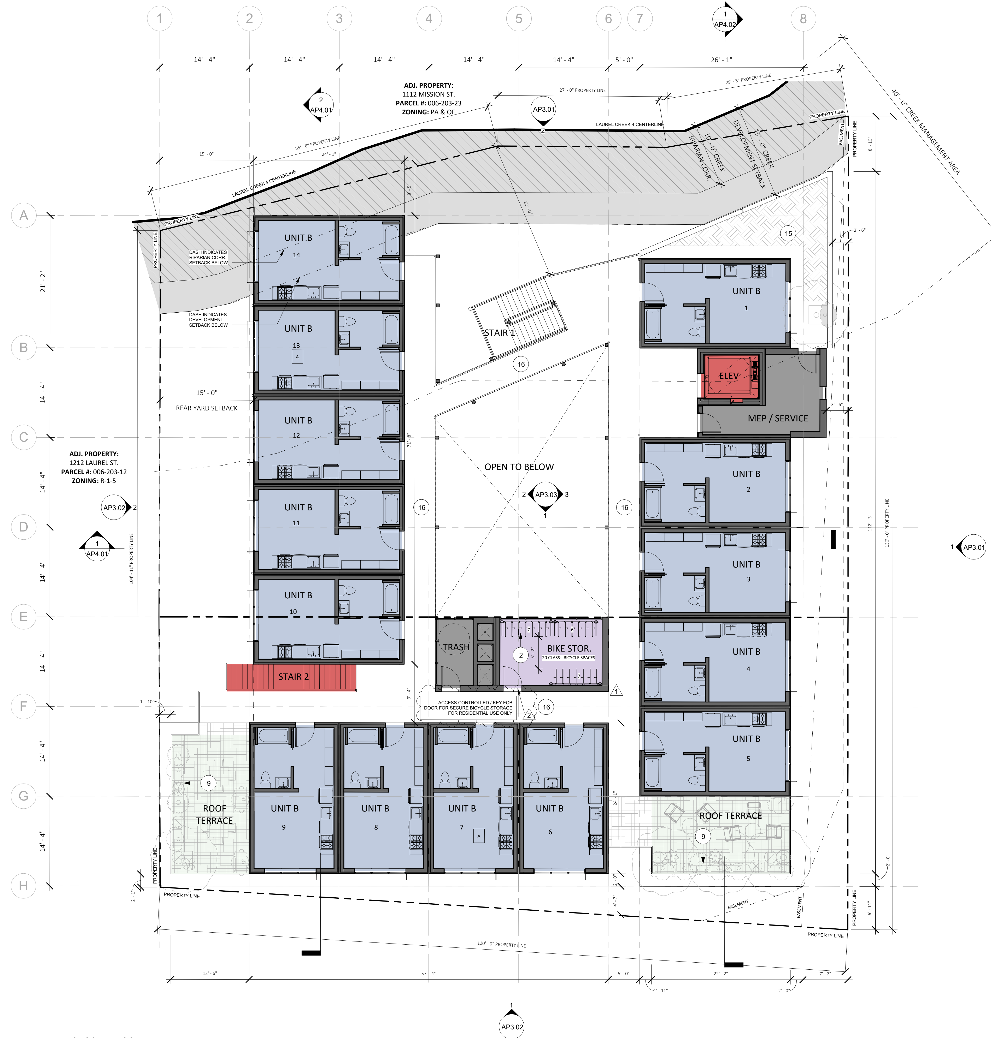
1 PROPOSED FLOOR PLAN - LEVEL 5 1/8" = 1'-0"
