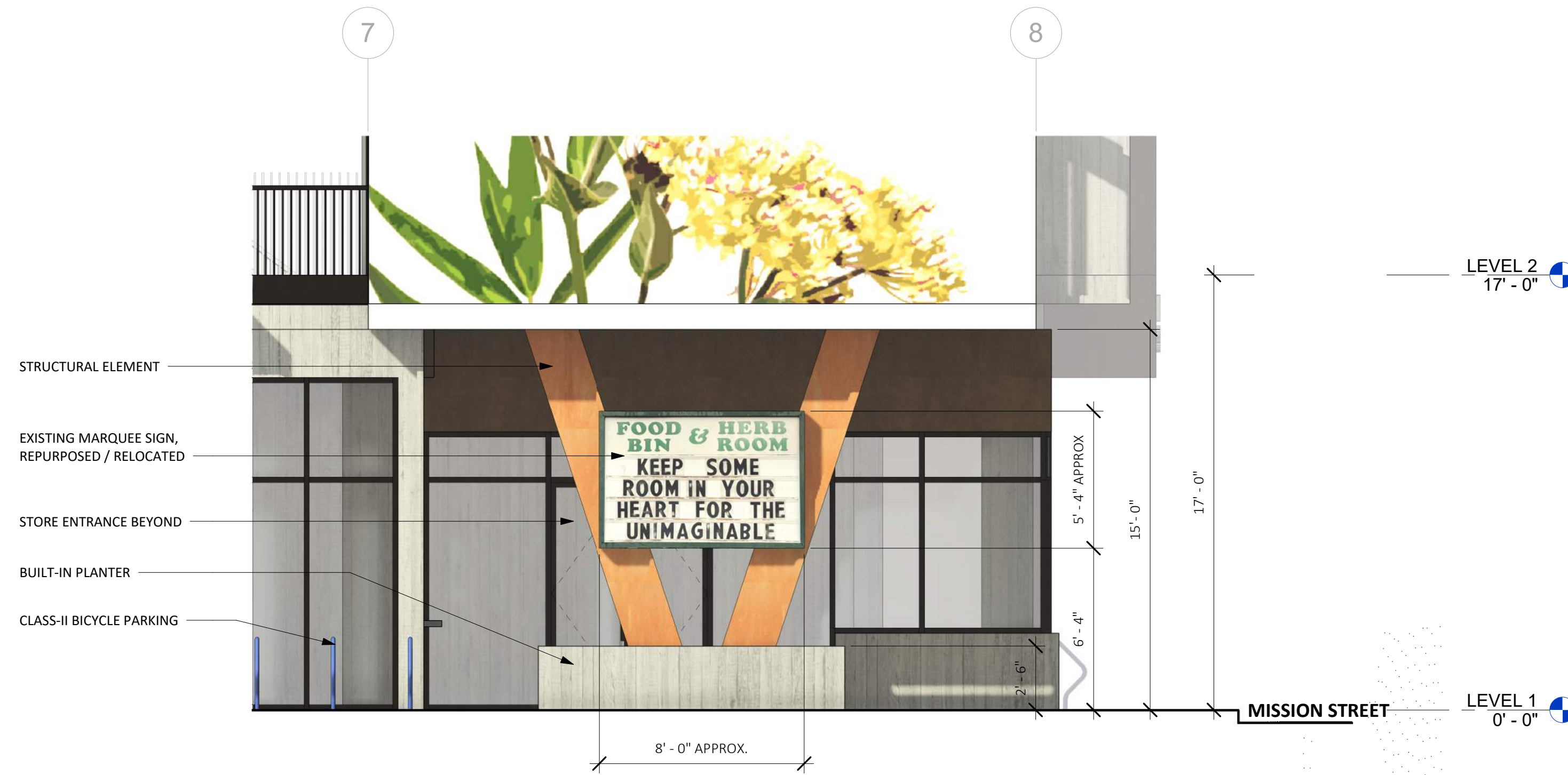
2 PROPOSED BUILDING SIGNAGE ELEVATION 1/4" = 1'-0"
