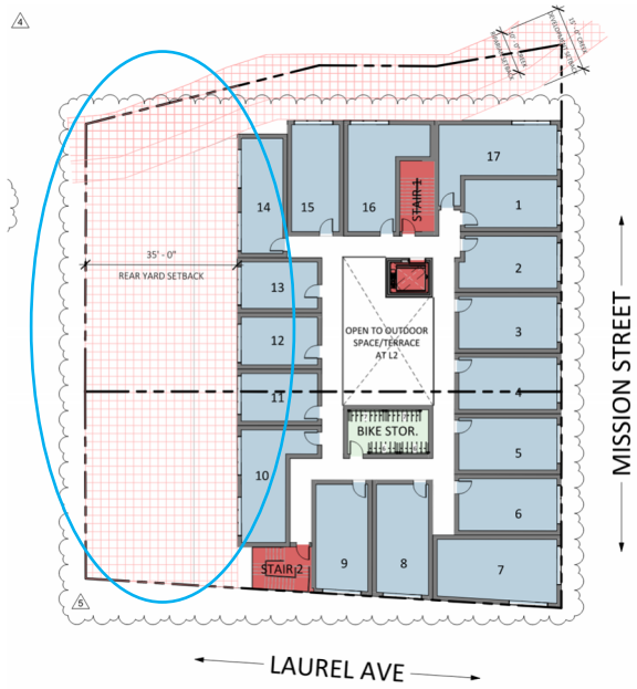
Planning Package Rev 5 – Updated base density diagram increasing RYSB from 15' to 35' at upper floors (NTS)
